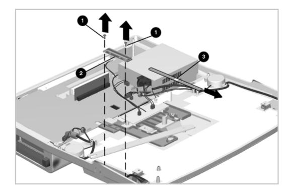
Figure 6-37. Removing the Docking Lever Cover
